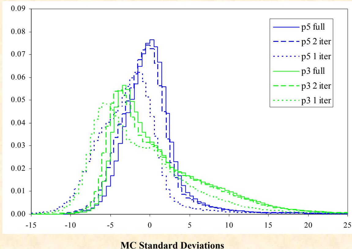
**Fractional Frequency Distribution of Voxel Energy Deposited Differences between Discrete Ordinates and Monte Carlo divided by MC Standard Deviation**
