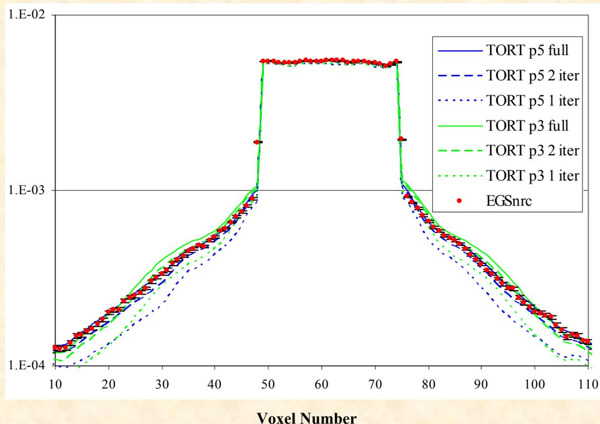
**Discrete Ordinates vs Monte Carlo Flux Transverse Profiles on a Mid-plane Coronal Slice halfway between CT Isocenter and Beam Exit**
