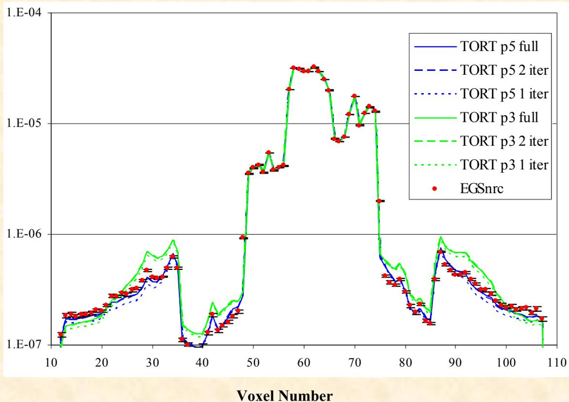
**Discrete Ordinates vs Monte Carlo Energy Deposited Transverse Profiles on a Mid-plane Coronal Slice halfway between CT Isocenter and Beam Exit**
